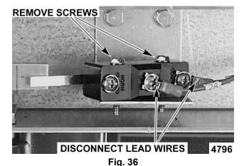
Reverse procedure to install the replacement switch and check for proper adjustment as outlined under DOOR SWITCH ADJUSTMENT.
